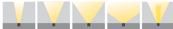
N: Narrow Angle M: Medium Angle W: Wide Angle XW: Without lens E: Elliptical Angle (60x120°)
