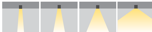
XN: Extra Narrow Angle N: Narrow Angle M: Medium Angle XW: Without Lens Angle
