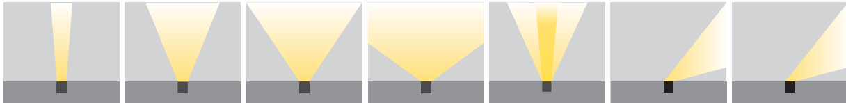
*XN: Extra Narrow Angle M: Medium Angle W: Wide Angle XW: Without lens *A: Asymmetrical *NA: Elliptical Narrow Angle *MA: Elliptical Medium Angle
