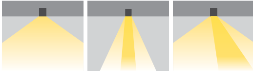
XW: Without lens A: Asymmetrical (60x120°) M3: 90x120°
