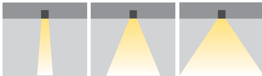
XN: Extra Narrow Angle M: Medium Angle W: Wide Angle
