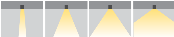
XN: Extra Narrow M: Medium Angle W: Wide Angle XW: Without Lens
